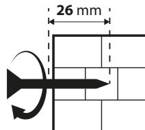
4. Insert the accessory anchors into the holes until they line up with the plane of the wall.
