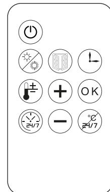
**Date setting:** After switching on, press the button and then use the + and - buttons to set the current date (eg. 01-07).
